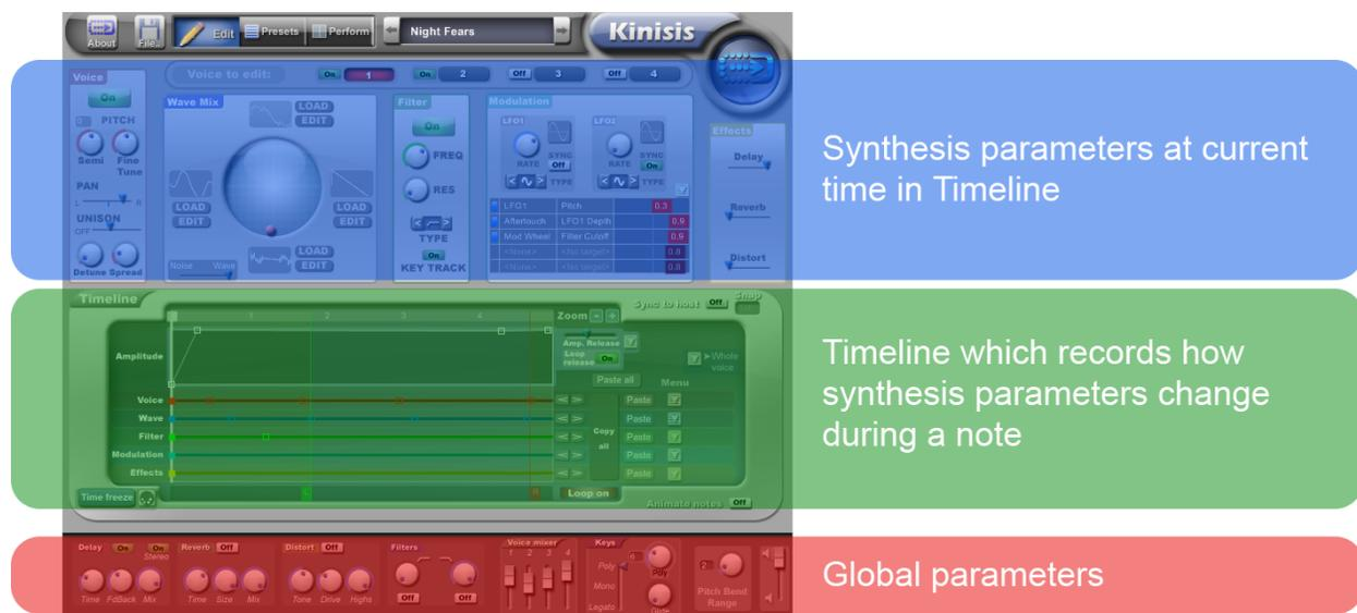
There are three main parts to the interface which have different roles. The **synthesis parameters** control what sound is produced *at the current point in the Timeline*. Note that this is different from normal synthesisers where knobs and sliders control the whole sound. In Kinisis, you are controlling a single time point in the note.
