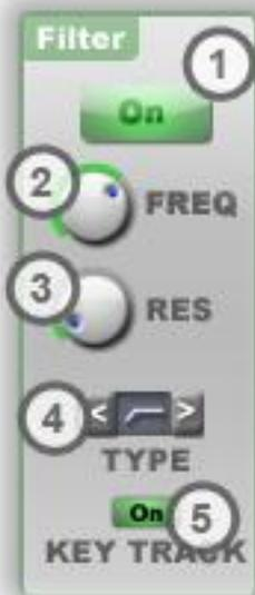
1) Turn the filter *on* or *off*. When *off*, the other controls in the filter section have no effect.
