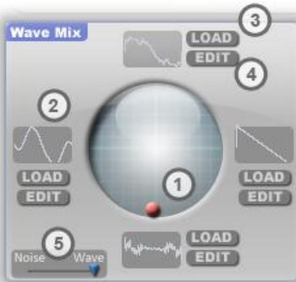
1) Mix between the four waves shown at the sides to produce the single wave that is played. Move the red dot closer to make it louder than the others. When the dot is centered, an equal mix of all four waves is produced.
