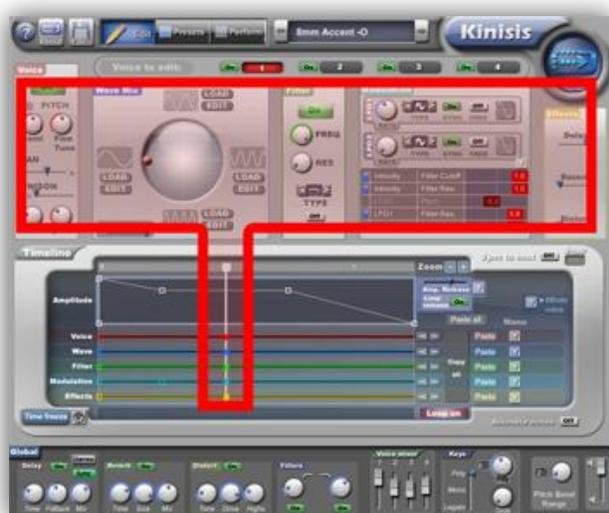
The synthesis controls at the top of the screen set move to show the values at the current point in the Timeline. Moving a control stores the value in the Timeline at the point being edited. A parameter can be made to change over time by moving to different points in the Timeline and setting values. Kinisis blends between the values as it moves
