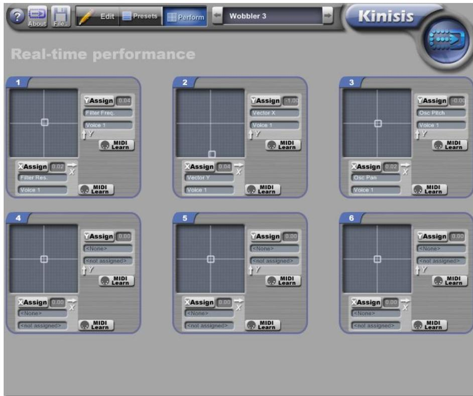
Six X-Y pads are provided, with 2 parameters assignable to each pad. Move the pointer around the pad to control a value, with the X axis (left-right) controlling one value, and Y axis (up-down) controlling another.
